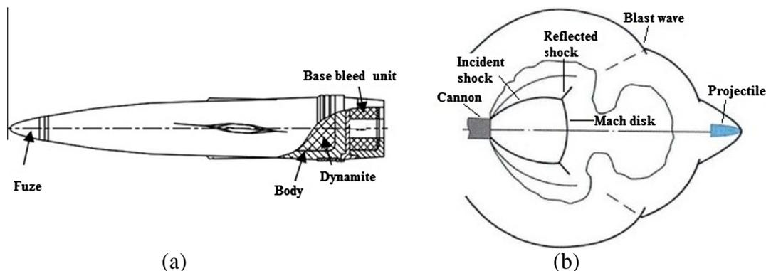
Fig. 1. (a) Schematic of base bleed projectile and (b) schematic of muzzle flows with moving projectile.
