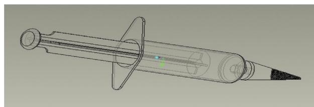
Fig. 1. Scheme of the novel HMIM microextraction device.
