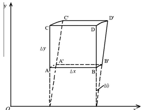
Fig. 1. Sketch of a control volume for axisymmetric problems,  $x, y$  are the axial and radial coordinate directions respectively.
