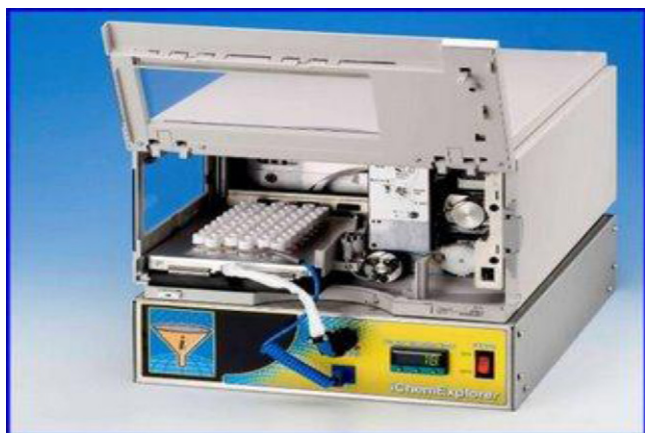
Fig. 1. The iChemExplorer (ICE) hardware, which includes a specially designed sample tray replacing the original sample tray of an Agilent (U)HPLC and a control unit installed directly under the Agilent (U)HPLC autosampler (courtesy of Reaction Analytics, Inc.).
