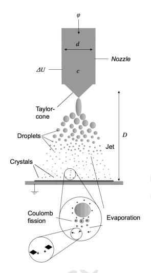
Schematic of the electrospray crystallization process. Using a small nozzle diameter (d), a low constant flow rate  $(\varphi)$ , relatively low solute concentration (c) a jet of highly charged small droplets will be emitted from the cone appearing at the nozzle tip when applying a high enough potential difference  $(\Delta U)$  at a certain working distance (D).
