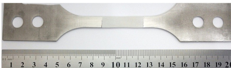
Fig. 2. The salt-coated creep specimen.
