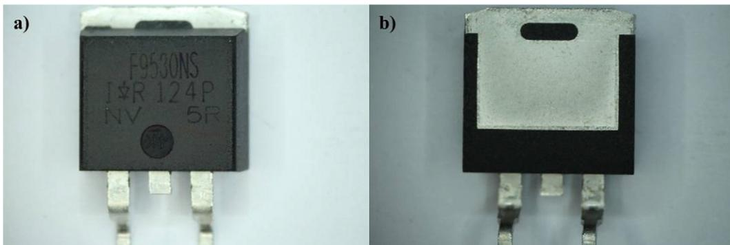
Fig. 2. Exterior view of the selected MOSFET: a) top view; b) bottom view.
