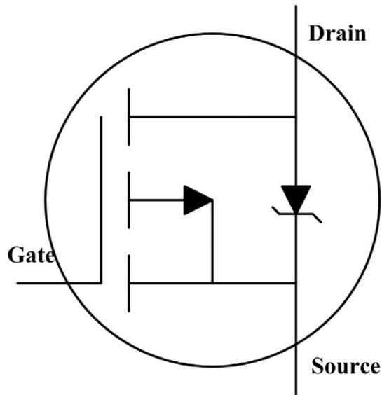
Fig. 1. Circuit schematic of the selected MOSFET.
