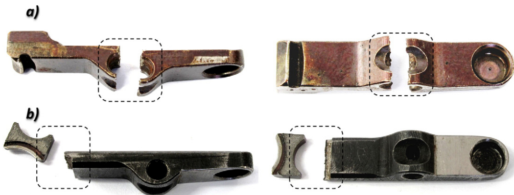
Fig. 1.1. The main view of MSBS extractor failures occurred during firing.
