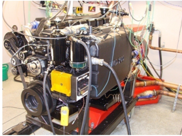
Fig. 1. Engine durability test setup.
