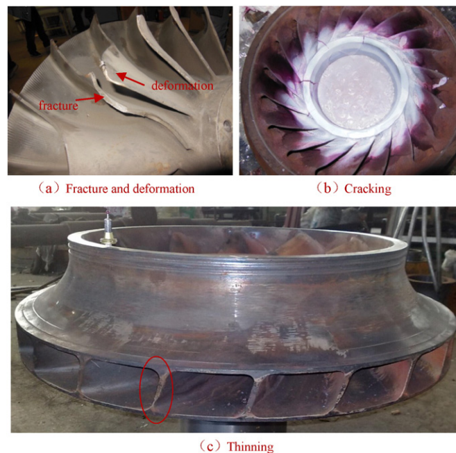
Fig. 1. The main failure modes of I&B.
