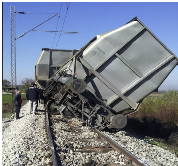
Fig. 1. Appearance of damaged railway car.
