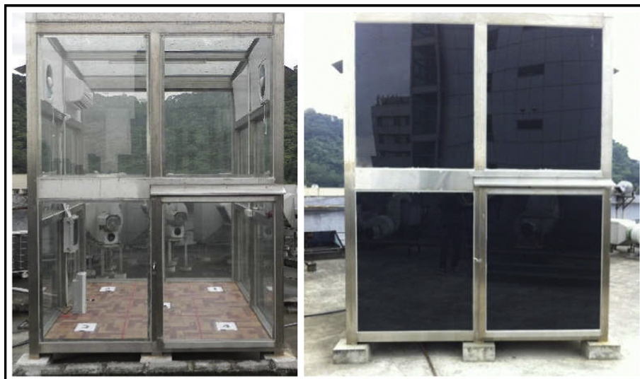
Fig. 2. Photograph of the ordinary glass (left) and HISG (right) curtain walls.
