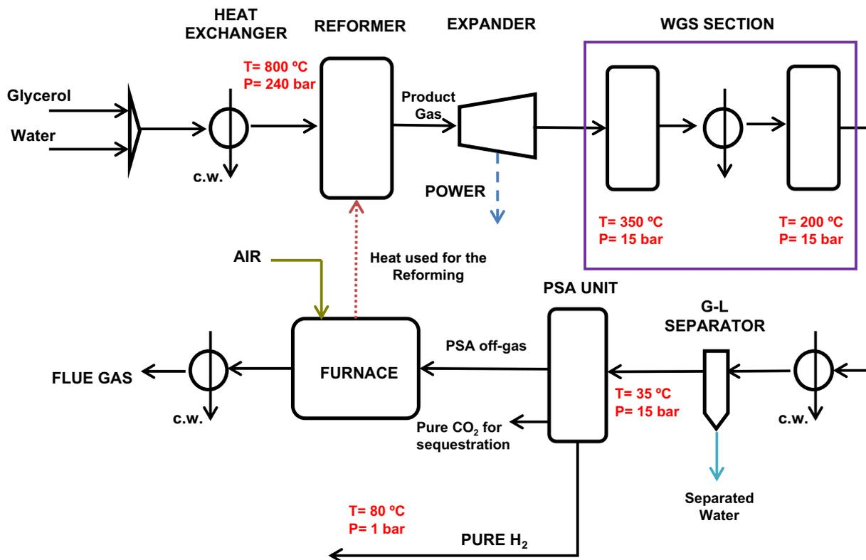
Fig. 1. Simplified flow-sheet of the supercritical water reforming process.
