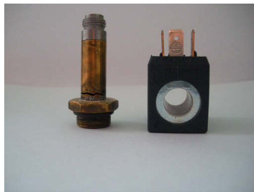
Fig. 2. Example of a fractured sleeve mounted on an electro-valve.
