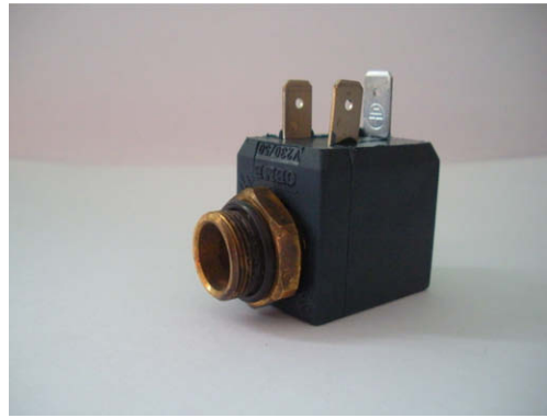
Fig. 1. An example of a whole electro-valve with the threaded brass sleeve.
