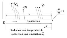
Fig. 1. Geometry of moving fin [14].
