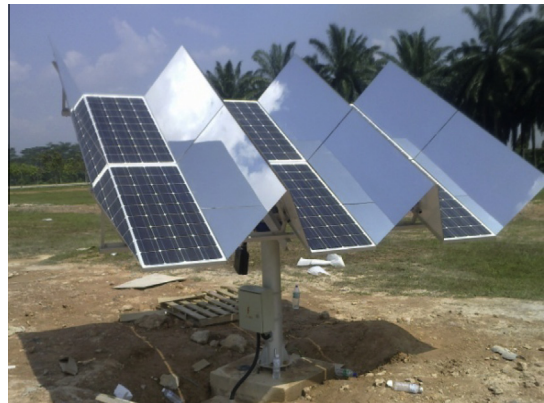
Fig. 1c. Installed CPV system with mirror concentrating elements.
