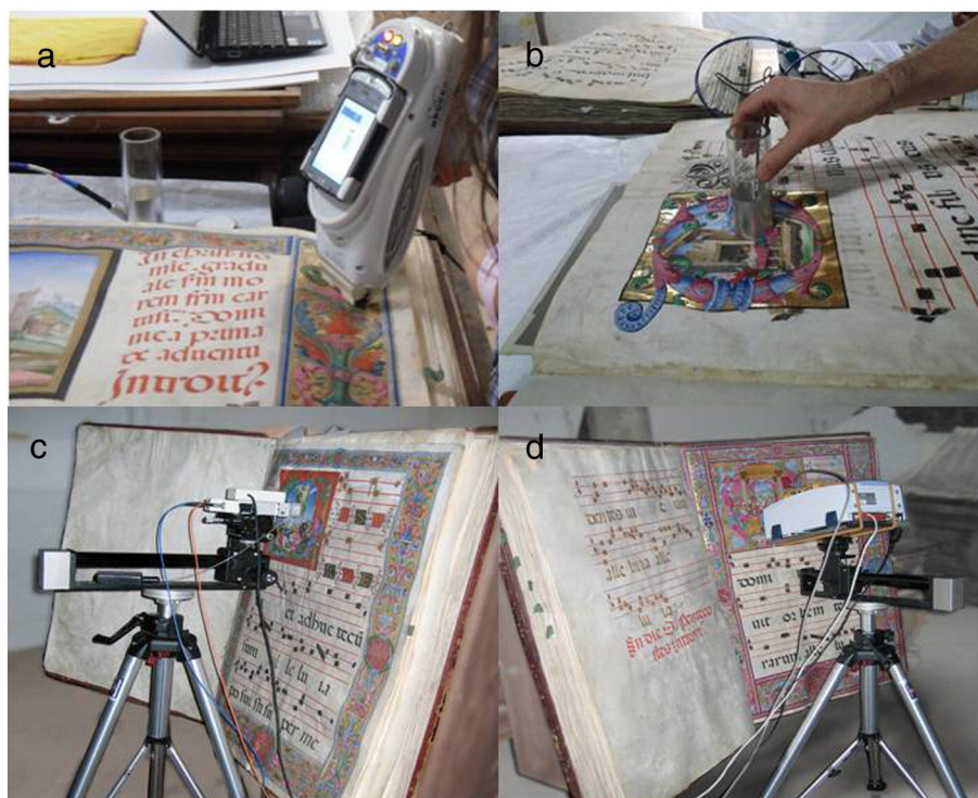
Fig. 1. The instruments at work in situ. (a) EDXRF instrument (Tracer III SD, Bruker); (b) Vis-NIR spectrophotometer (HR4000, Ocean Optics); (c) FTIR spectrophotometer (Alpha, Bruker); (d) Raman micro-probe (Jasco RMP-100 probe interfaced to a Lot-Oriel MS125 spectrometer).
