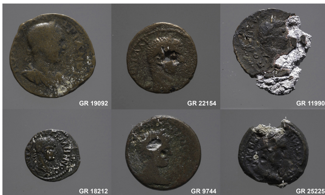
Fig. 2. Different grades of typical corrosion phenomena visible on Greek imperials.
