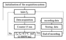
The program automatically opens an excel file; this file shows instantaneous values as ambient temperature  $T_a$ ; collector inlet, outlet, difference and mean water temperature; solar radiation G (W/m<sup>2</sup>), the collector efficiency.
