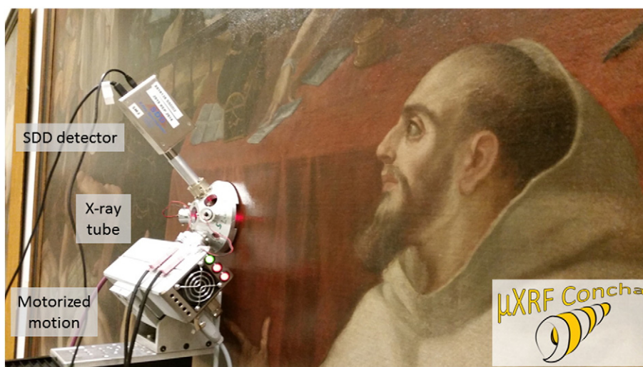
Fig. 2. General view of the \mu XRF-CONCHA setup doing in situ analysis of “San Pedro Nolasco despidiéndose de Jaime I El Conquistador.”
