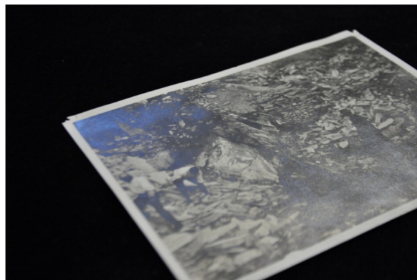
Fig. 2. Photo No. 1 – detail of the silver mirroring in the upper left corner.
