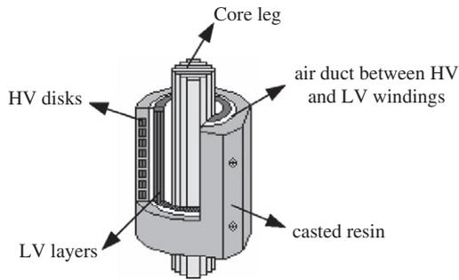
Fig. 1. Schematic view of cast resin transformer.
