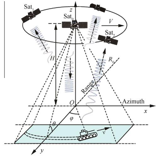
Fig. 1 Scene of spaceborne multistatic SAR surveying ground moving targets.
