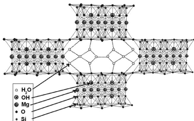
Fig. 1. Sepiolite structure: projection onto the (001) plane.
