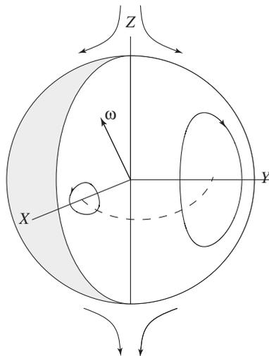
**Fig. 1.** Schematic view of the unperturbed flow. Vector  $\omega$  denotes the external vorticity. Two characteristic streamlines are shown. The dashed line is the circle of degenerate elliptic fixed points.
