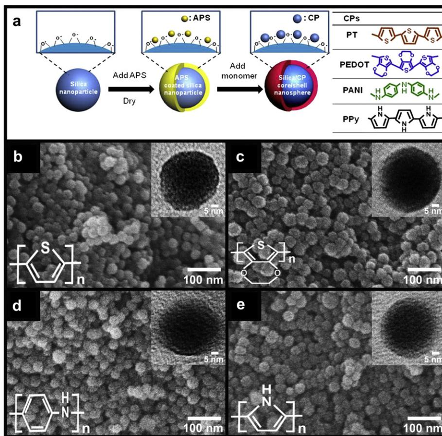
**Fig. 1.** (a) Schematic diagram for fabrication procedure of silica/CP core/shell NSs; SEM images of silica/CP core/shell NSs prepared via seeded polymerization (insets: TEM images of a corresponding single core/shell nanosphere. Scale bars = 5 nm); (b) PT, (c) PEDOT, (d) PANI and (e) PPy. Scale bars = 100 nm.
