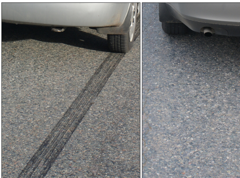
Fig. 1. Braking tracks from car without ABS (left) and with ABS (right). The braking tracks were made from initial speed 58 \text{ km} \cdot \text{h}^{-1} to complete halt by using maximum braking effect.
