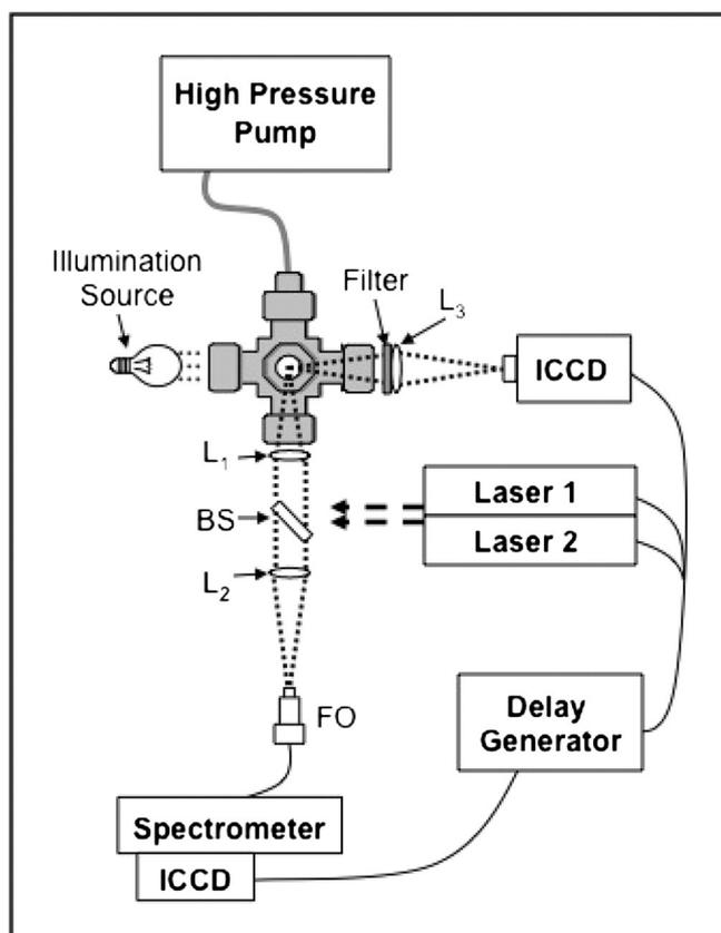
**Fig. 1.** Schematic diagram of LIBS spectrographic and shadowgraphic apparatus. The two laser beams were collinearly aligned along the same path. The labels L, BS, and FO indicate lens, beamsplitter, and fiber optic, respectively.
