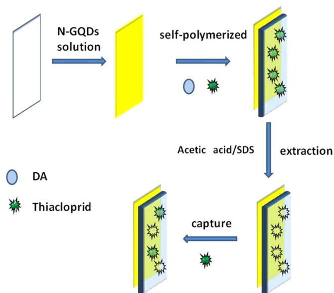
Scheme 1. The process of the molecularly imprinted N-GQDs based fluorescence strip preparation.
