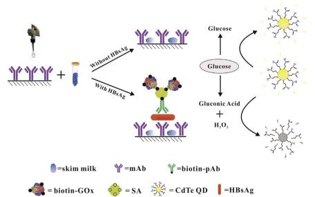
**Scheme 1.** Schematic of fluorescence ELISA based on GOx-induced fluorescence quenching of MPA-ODs for HBsAg detection.
