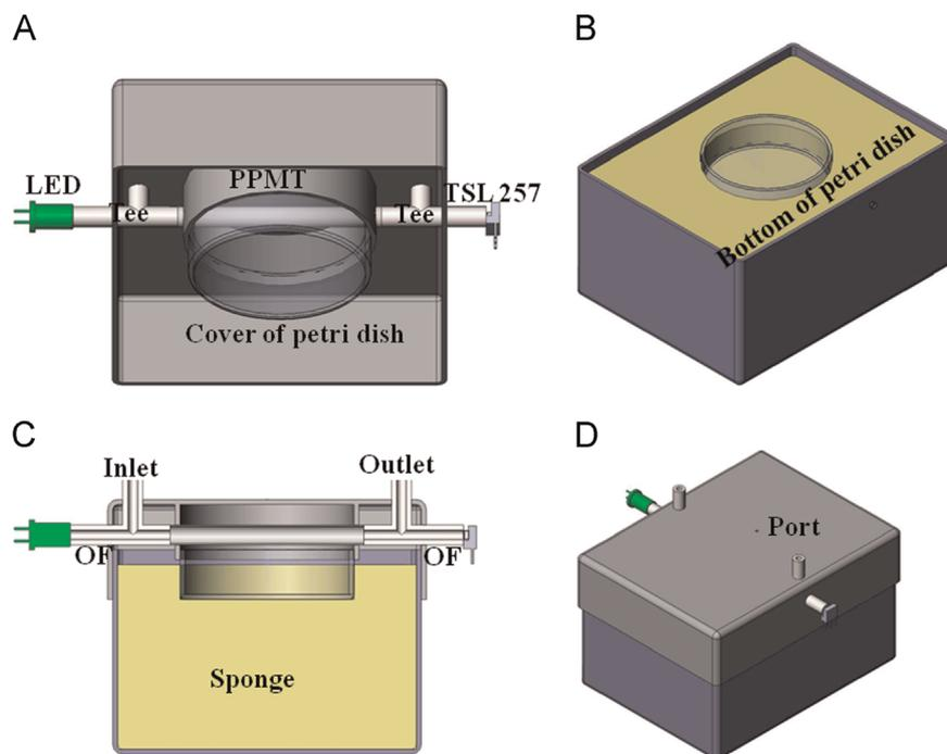
**Fig. 1.** Schematic diagram of sulfide measuring device. (A) Top cover of the device; (B) bottom of the device; (C) section view of the device; (D) integral exterior of the device. LED: light emitting diode; TSL257: TSL257 light-to-voltage converter; PPMT: porous polypropylene membrane tube; and OF: optical fiber.
