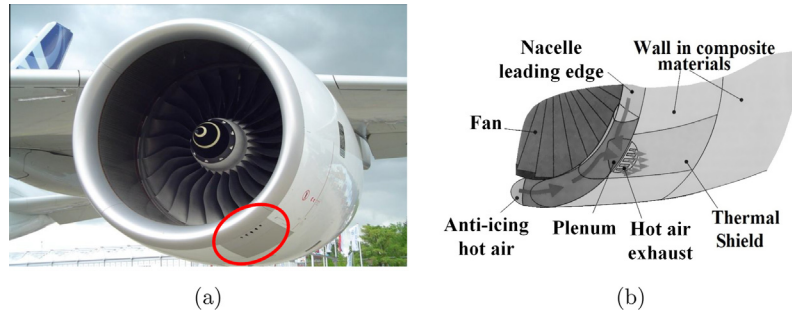
Fig. 1. (a) Hot air exhaust from the anti-icing system on a A380 engine. (b) The different components of the anti-icing system.
