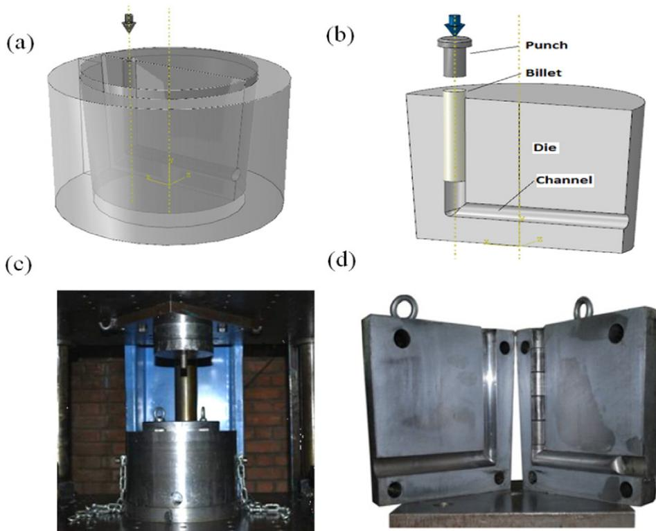
Fig. 1. (a) 3D view of the ECAP die, (b) cross-section of the die, (c) die ready for ECAP and pressing and (d) ECAP-processed sample inside the die [7].
