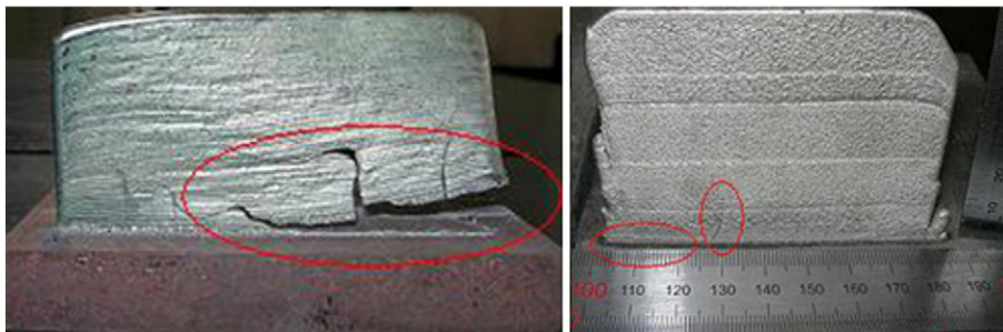
Fig. 1. Cracked thin-wall metal parts fabricated by LDDS.
