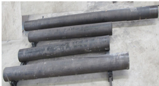
Fig. 2. The drill pipe specimens.
