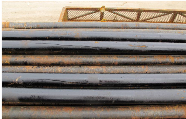
Fig. 1. Visual inspection of axial cracking drill pipes.
