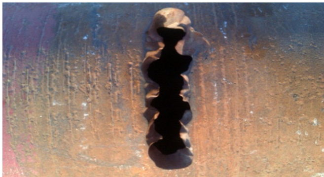
Fig. 1. Slip-cuts on 5" DP resulting in a wash-out.
