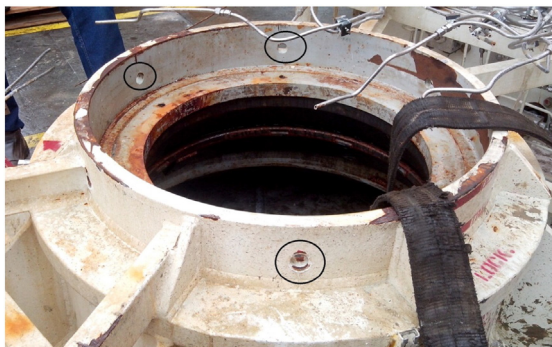
Fig. 2. Tree cap after re-motion – the location of three screws is indicated by circles.
