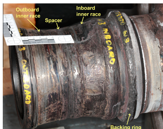
Fig. 1. Catastrophic bearing failure. (a) Condition of the bearing on the axle shaft after the outer ring was removed.
