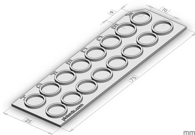
Fig. 1. Isometric schematic of 16-well nylon-based plastic slide.
