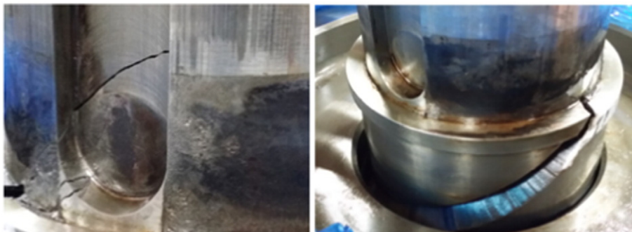
Fig. 2. Torsional fatigue failure of the shaft.
