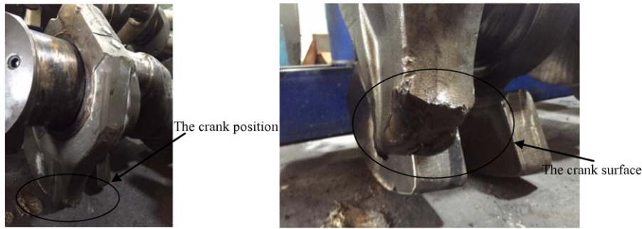
Fig. 1. The failed connecting rod.
