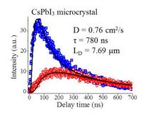
Carrier diffusion and recombination kinetics in all-inorganic CsPbI<sub>3</sub> perovskite microcrystals directly synthesized in solution phase are reported.
