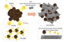
We report a "soft" graphene oxide-organopolysulfide nanocomposite with improved *pseudo*capacitive performance for high-potential (1-2.8 V vs. Li<sup>0</sup>/Li<sup>+</sup>), high-capacity (278 mA h g<sup>-1</sup>) and stable (500 cycles) lithium storage.
