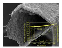
The vertical crosslinking MoS<sub>2</sub>/three-dimensional graphene composite has been prepared by hydrothermal method, which delivered a superior and stable electrochemical capacitive performance.
