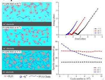
Temperature stability of symmetric activated carbon (AC) supercapacitors (SCs) assembled with *in situ* electrodeposited poly(vinyl alcohol) potassium borate hydrogel electrolyte was systematically studied and compared with that of AC SCs assembled with liquid aqueous electrolytes in the temperature range from -5 °C to 80 °C.
