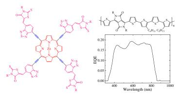
A star-shaped electron acceptor with porphyrin as core and rhodanine-benzothiadiazole as end groups linked with ethynyl units was developed for non-fullerene solar cells, in which a PCE of 1.9% with broad photo response was achieved when combining with a diketopyrrolopyrrole-polymer as electron donor.
