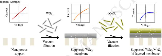
Through a two-step vacuum-filtration process, WSe<sub>2</sub> and MoS<sub>2</sub> nanosheets were sequentially deposited onto a polymeric nanoporous support, forming WSe<sub>2</sub>/MoS<sub>2</sub> bi-layered heterostructure. Highly rectified ion transport phenomenon is observed through the heterogeneous 2D layered membranes.
