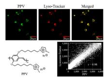
A cationic poly(p-phenylenevinylene) derivative (PPV) is designed and synthesized to bear quaternized N-methyl-imidazole groups, which is successfully utilized in lysosome-specific and long-term imaging.
