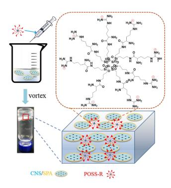
A novel kind of inorganic-organic hybrid supramolecular hydrogel with excellent anti-biofouling capability was developed. The hydrogel was formed via ionic interaction between the negative-charged sodium polyacrylate (SPA) entwined clay nanosheets (CNS) and positive-charged polyhedral oligomeric silsesquioxane (POSS) core-based generation one (*L*-Arginine) dendrimer (POSS-R).
