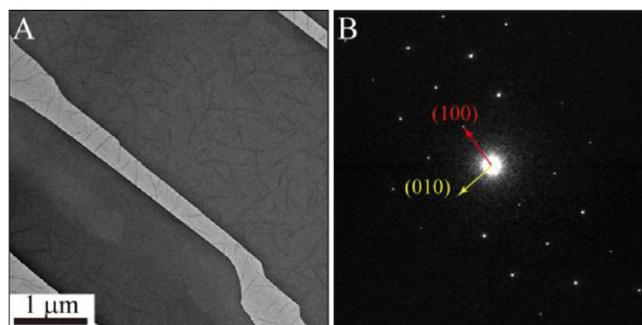
**Fig. 2.** (A) TEM image showing the coexistence of nanofibers and single crystals (dark ribbons). (B) SAED pattern showing the single crystallinity.
